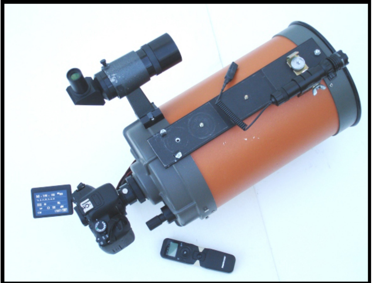
PHOTO #3 Canon EOS T4i with Celestron C8 2000mm f 10, top of tube has bracket to mount other equipment.
