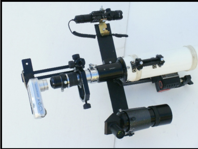
PHOTO #1 Sony DSC-P200 with Unitron 900mm f 15 refractor. Orion camera bracket, eye pieces as needed, green laser pointer at top with on-off switch cable and finder scope at bottom.
