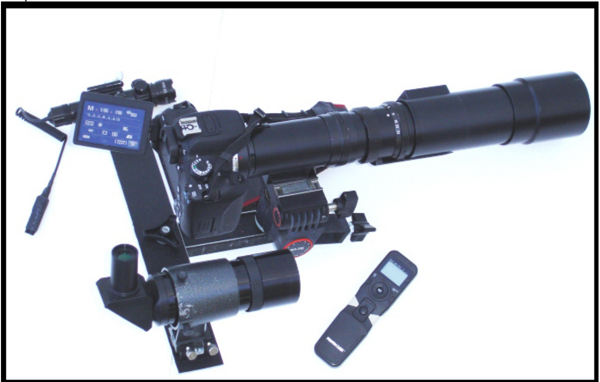
PHOTO #2 Canon EOS T4i with 400mm f 6.8 telephoto, see adjustable viewing screen, remote switch (or interval timer) and tripod head on dovetail bracket under the lens.
