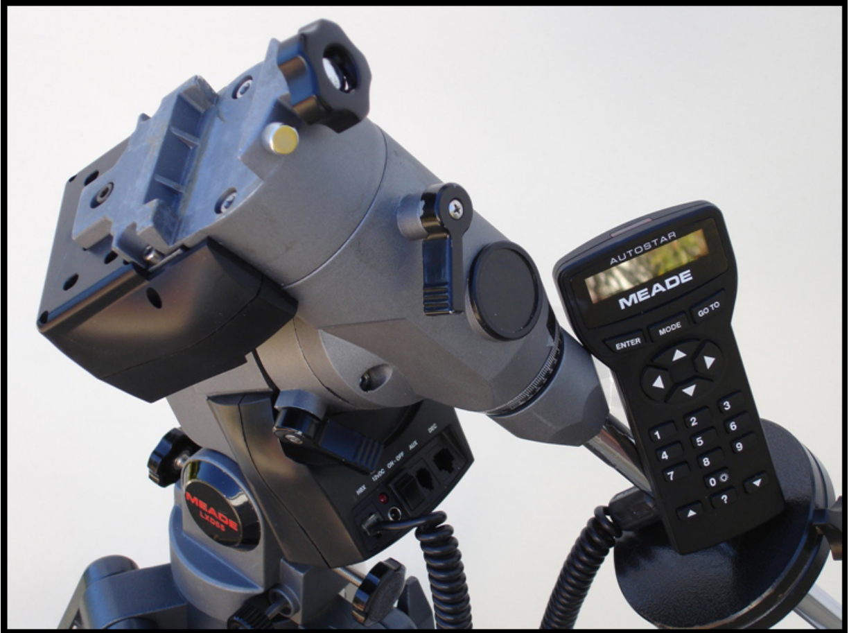
PHOTO #4 Meade LX200 German Equatorial mount. See dovetail groove at top left. The remote hand controller helps in tracking the objects in the night sky.
